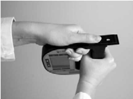
Fig. 12 - 3 Removing the pump lock
