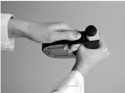
Fig. 12 - 1 Removing the pump
