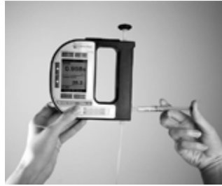
Fig. 10 - 2 Filling sample using the plastic syringe
