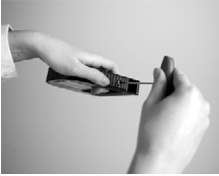
Fig. 12 - 2 Removing the pump lock screw
