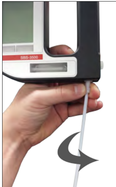
Fig. 7 - 1 Connecting the filling tube
