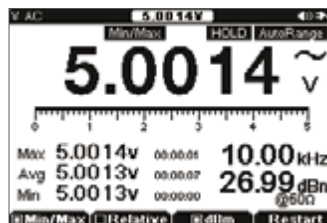
Voltage data logging screen shot
