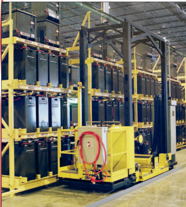
Triple stacking system featuring a PCE-2-32-TS-V-SG
