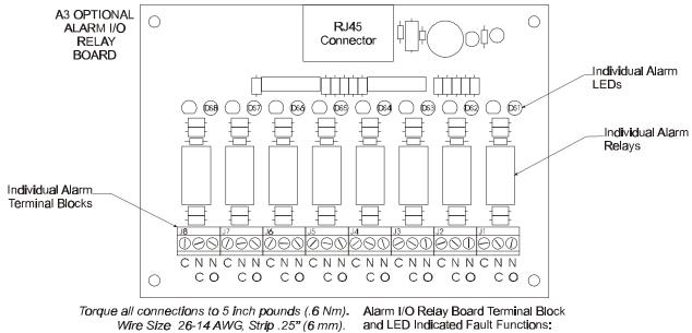
Terminal Block LED Fault Functions Key: C= Common
