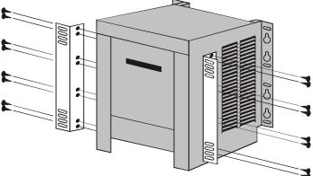
ACAUTION: TO ENSURE THE STRUCTURAL INTEGRITY OF THE RACK MOUNTING BRACKETS, USE THE SIXTEEN #10 SELF-THREADING SCREWS PROVIDED IN THE KIT. USE EIGHT SCREWS PER BRACKET AND TIGHTEN THEM UNTIL SNUG. DO NOT STRIP THE THREADS.
