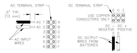
AWARNING: IMPROPERLY CONNECTED WIRING CAN CAUSE AN ELECTRICAL FIRE.
