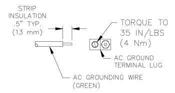
AWARNING: DO NOT OPERATE THE CHARGER WITHOUT PROPER GROUNDING. IMPROPER GROUNDING MAY CAUSE AN ELECTRIC SHOCK, WHICH COULD RESULT IN INJURY OR DEATH.
