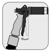
Squeeze the trigger to clear the hose of any air.
