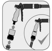
Attach the quick-connect fitting and the gun to your 1/2" (12.5 mm) water hose.
