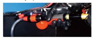
3. Watch the spinner mounted on the Instant Valve Pro. When it stops spinning, the filling is completed (about 15 seconds, usually).
