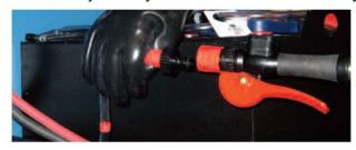
Squeeze the lever completely to fill the battery.Do Not Partially Squeeze the Lever.
