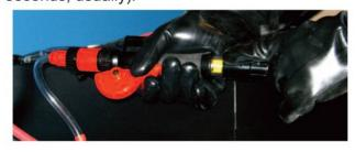
4. Release the lever and then disconnect the Instant Valve Pro from the Water Injector System.
