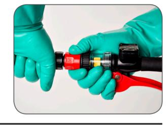
When filling operations are complete, turn the inverter off and store the red output hose. If the tank is going to remain unused for an extended period of time, drain the tank.
