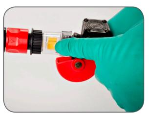
Watch the spinner mounted on the Instant Valve Pro. When it stops spinning, the filling is completed (about 15 seconds, usually). Release the lever.
