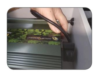
NOTE: Inverter will shut off when battery voltage reaches 12.5VDC. If this occurs, fully charge the battery before the next use.
