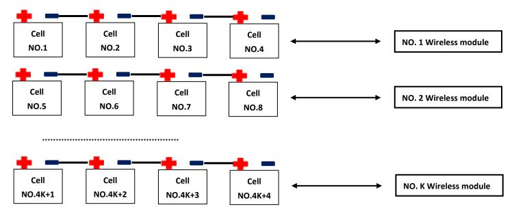
4.4.1.1 Reading the module number from the modules' labels, find the correct cells to connect the module to. Do not connect the modules to 4 batteries which are not in series like No. 1, 5, 8, 9 - misconnection will likely damage the module immediately!
