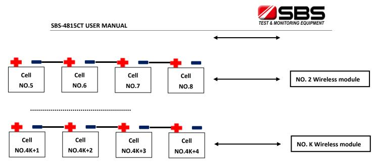
4.4.3.1 Read the module number from the label the modules, find the correct cells to connect the module to. Do not connect the modules to 4 batteries which are not in series like NO. 1, 5, 8, 9 – the misconnection will likely damage the module immediately!
