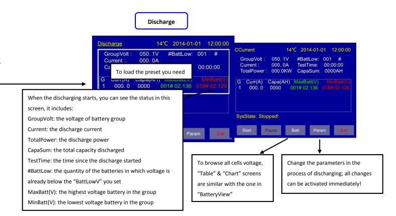
4.8.6 Press "Param" to adjust the parameters during the discharge (if necessary); all changes can be activated immediately and the discharge will not be stopped.
