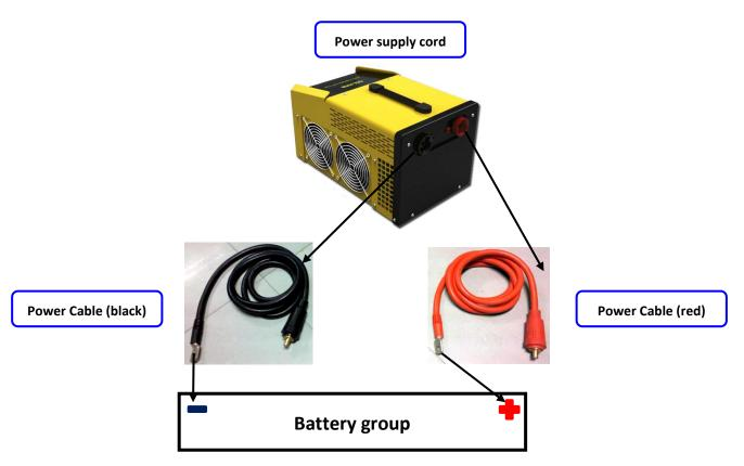
4.3.1 Use the power cables (1 red, 1 black) to connect the main machine with the battery string being tested.
