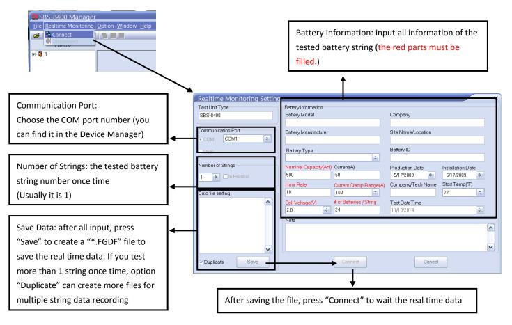
5.3.3 Start the discharge on the SBS-4815CT, and the real time data will keep coming and showing in the PC software interface. Please input the red parameters correctly in the battery information, it can affect the result of capacity evaluation.
