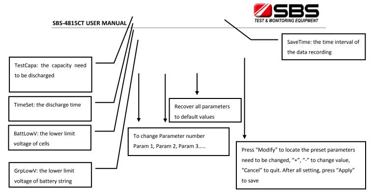
**4.7.2** "TestCapa", "TestTime", "BattLowV", "GrpLowV" are the test stop conditions, if any of these set-points is reached, the discharge will stop automatically.
