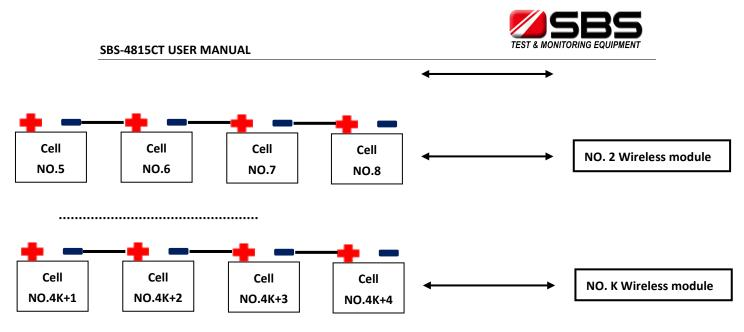
4.4.2.1 Read the module number from the label in the modules, find the right batteries to connect with. Do not connect the modules to 4 batteries no adjacent like NO.1,3,8,9, it will probably damage the module immediately!
