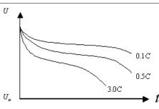
We know for different types, materials and craftwork, the voltage dropping data is the most uniform and accurate evident for estimating the battery capacity. The curve not only shows this information, but also shows that using different hour rates to discharge the same batteries would yield different results. To avoid the harm of discharging, your discharge has to apply the suitable hour rate.
