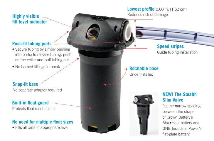
The Stealth Watering System<sup>™</sup> is a float-based, single-point watering system that precisely fills all battery cells to the same level simultaneously. Watering batteries with the Stealth Watering System is safe, easy and affordable – and takes one tenth the time of hand watering. It is perfect for installations of 5 to 25 batteries and is best used with conventional charging applications.
