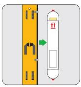
Remove cartridge from the mounting plate to ease installation.
