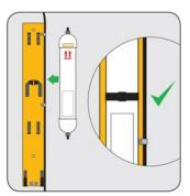
Re-attach the cartridge to the mounting plate using the strap. Ensure arrows are pointing up.
