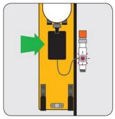
Attach the battery case firmly to the velcro strips on the backplate.
