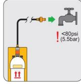
Connect the free end of the black inlet hose to the water supply.
