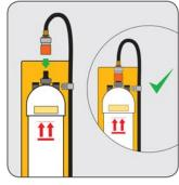
Connect the fixed end of the black inlet hose to the cartridge.
