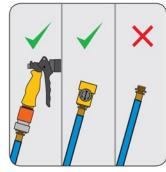
Attach either the **Watering** *Gun* or Flow Restrictor to the free end of the blue hose.
