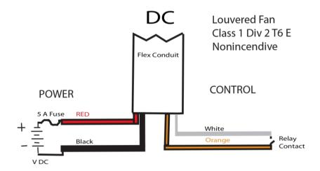
The flexible shielded electrical conduit contains four wires. Red(+) and Black(-) are for connection to DC power. See the data plate on the fan for the appropriate voltage. The other two wires are Black and Orange and connect to a normally open switch or relay contacts. Contact closure activates fan.
