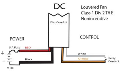
The flexible shielded electrical conduit contains four wires. Red(+) and Black(-) are for connection to DC power. See the data plate on the fan for the appropriate voltage. The other two wires are Black and Orange and connect to a normally open switch or relay contacts. Contact closure activates fan.
