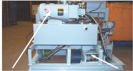
Hydraulic Power Unit
